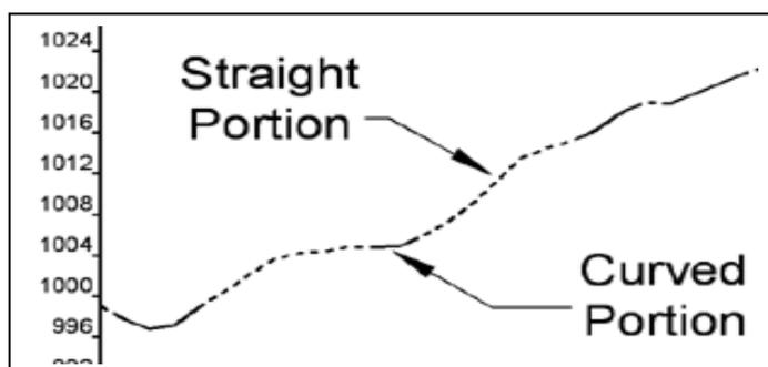
Figure 6. Finished horizontal alignment in long section for easy establishment of coordination between horizontal and vertical alignment.
